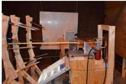
Side view photograph showing the concave pressure probe array.
