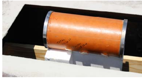
b) Casing with steel particle liner aligned with test plane
