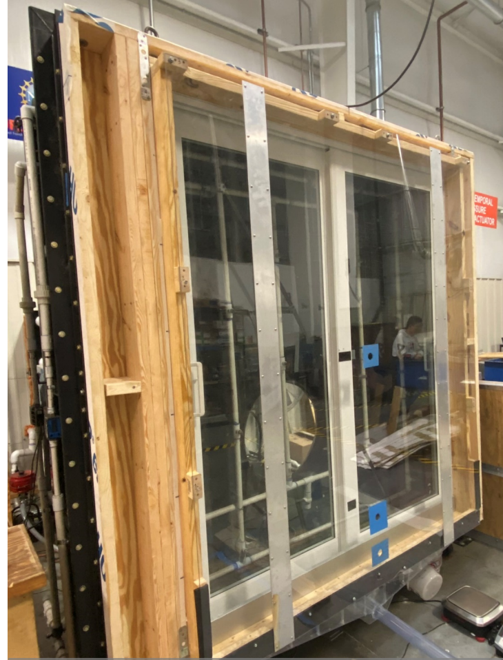
Sliding Door Installation on HAPLA Face with Protective Viewing Panel
