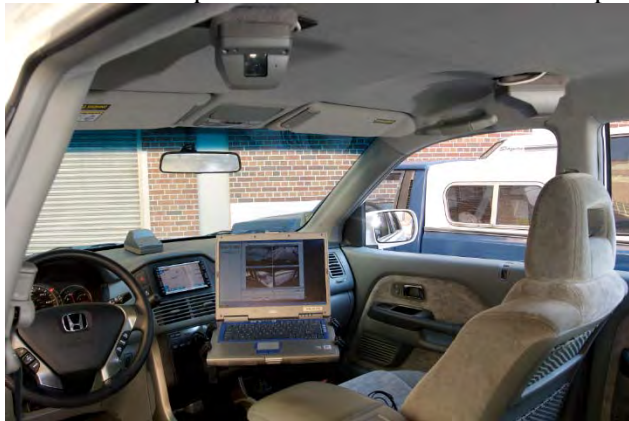
Figure 35: Inside View of the TRC Instrumented Vehicle
